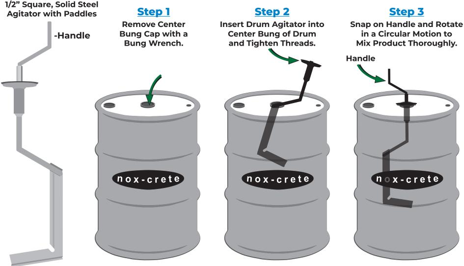
**NOTE:** Always Replace Drum Bung Cap Immediately After Mixing And Never Leave Drum Open.
