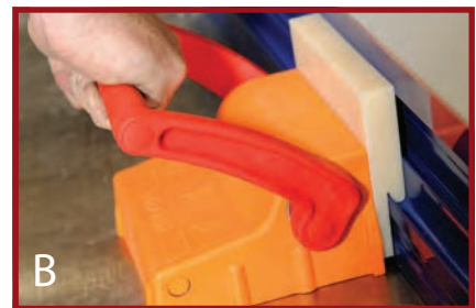
TITAN™ MAGNET CLAMP IS PARTIALLY ENGAGED.
