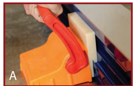
TITAN™ MAGNET CLAMP IS FULLY DISENGAGED.
