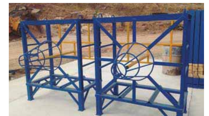
Storage box for tensioning strands
