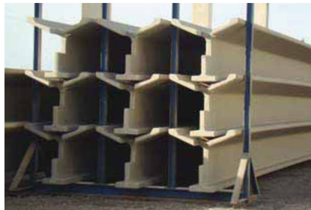
Ypsilon roof girders
