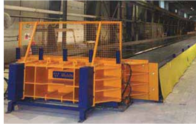
Self supporting TT mould for roofs or pre-slabs of industrial and commercial buildings such as parking garages.
