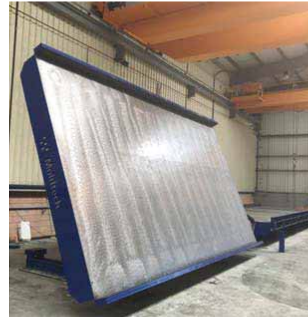
Tilting table with polished surface
