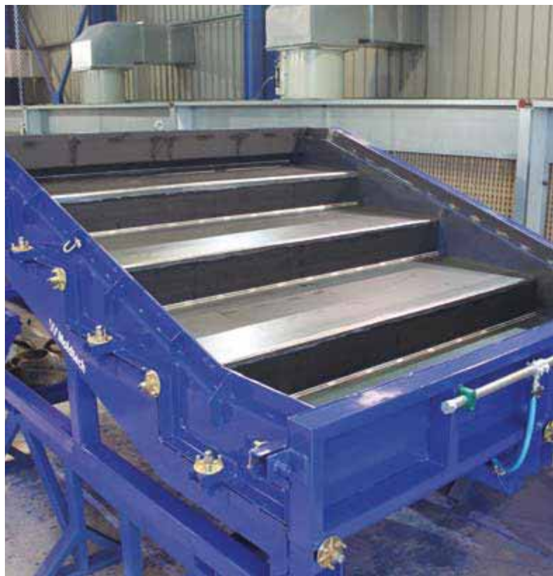
Mould for grandstands
