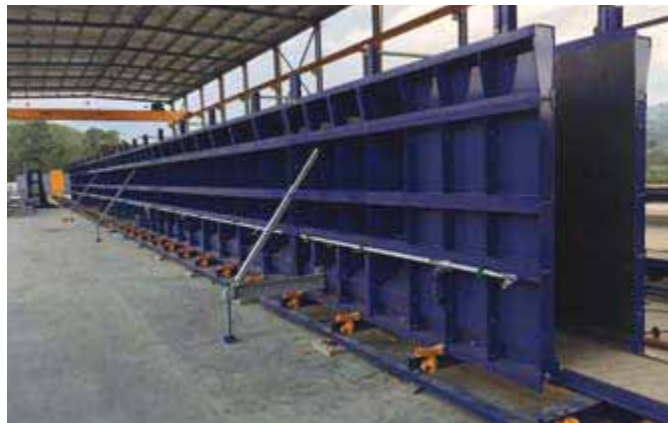
'I' beam mould on casting bed
