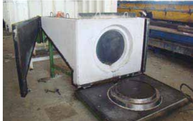
Mould for wing walls
