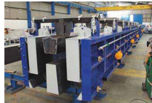
Mould sides for "H" beam used as water channel
