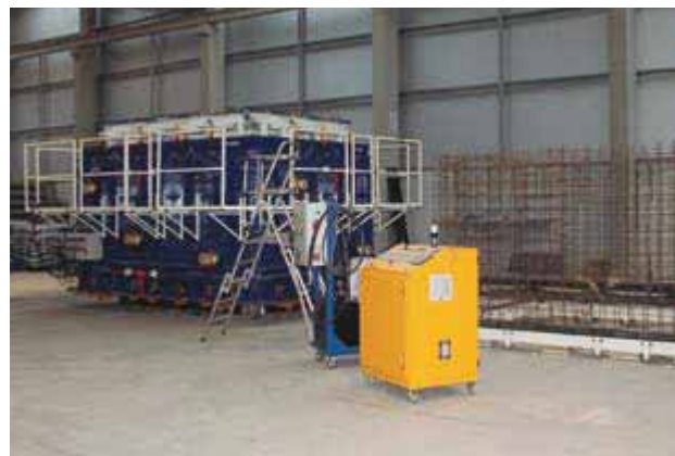
MT20 mould with hydraulic unit and control panel for electrical vibration.
