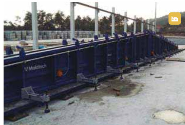
Delta beam mould on self-supporting bed
