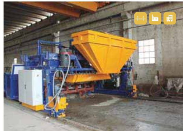
Casting bed cleaning machine
