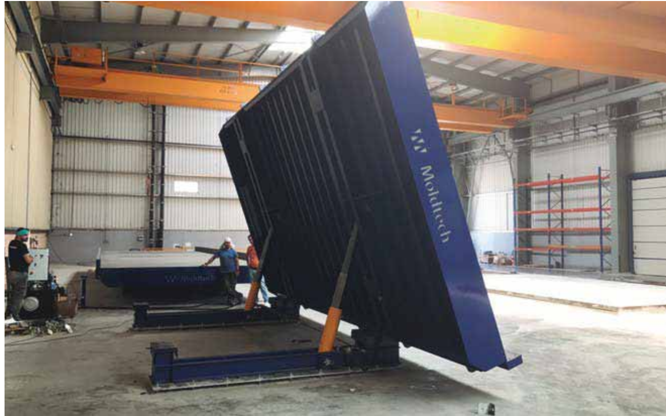
Tilting table 12 x 4.5 meters with capacity of 600 kg/m2
