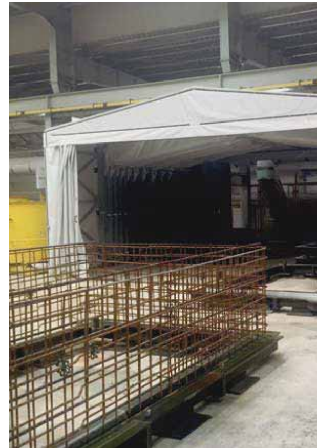
MT20 baseplates, ready with reinforcement.
