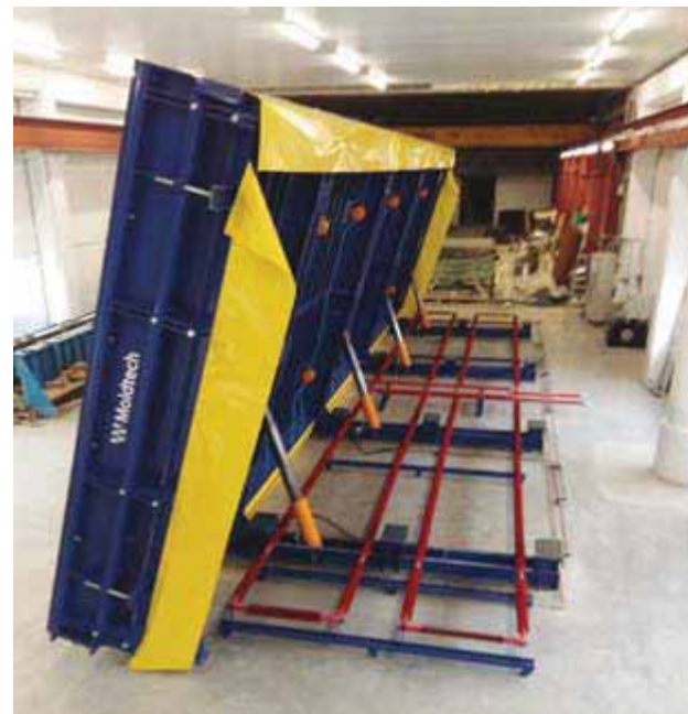
Detail of tilting table with polished surface
