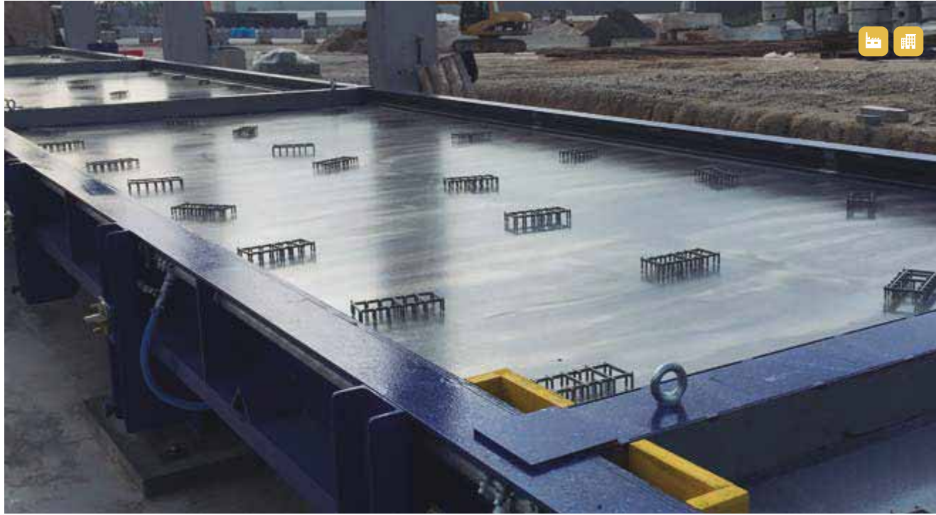
Tilting table with polished surface
