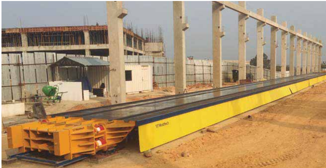
Self supporting TT mould for roofs or pre-slabs of industrial and commercial buildings such as parking garages.
