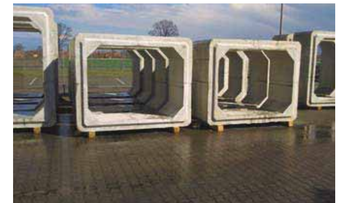
Precast box culvert after removing MT20 inner and outer moulds.
