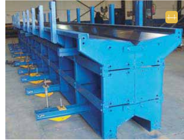
Sides for bridge girder
