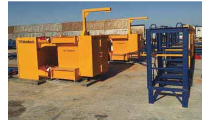
Storage boxes for tensioning strands
