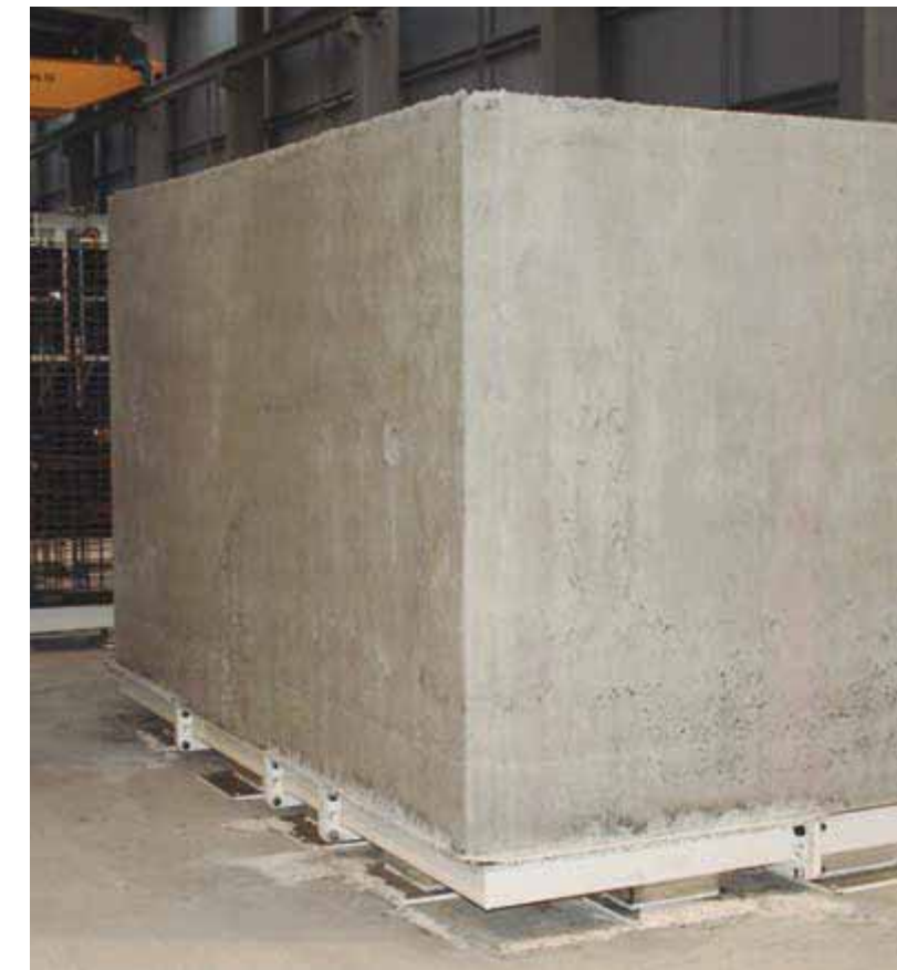
Precast box culvert after removing MT20 inner and outer moulds.
