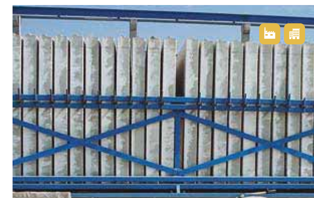
Storage rack for panels
