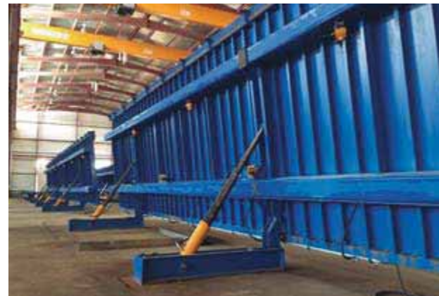
Venezuela: complete installation for the production of 3.000 precast housing units per year, using tilting tables of 15.5 x 3 meters
