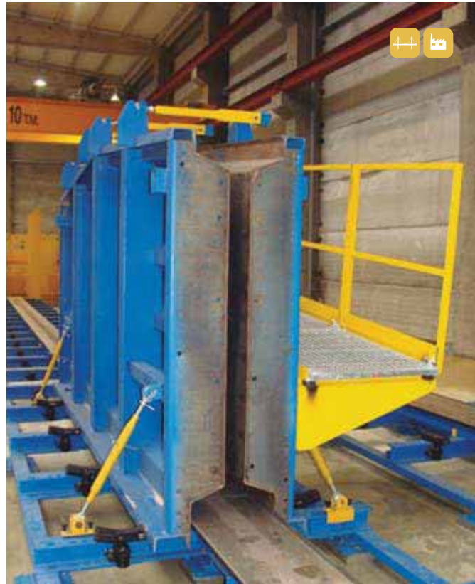
Detail of casting bed system
