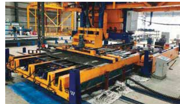
Moulds at filling station
