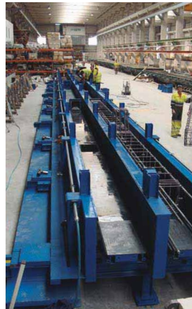
Hydraulic double mould for columns prepared with reinforcement
