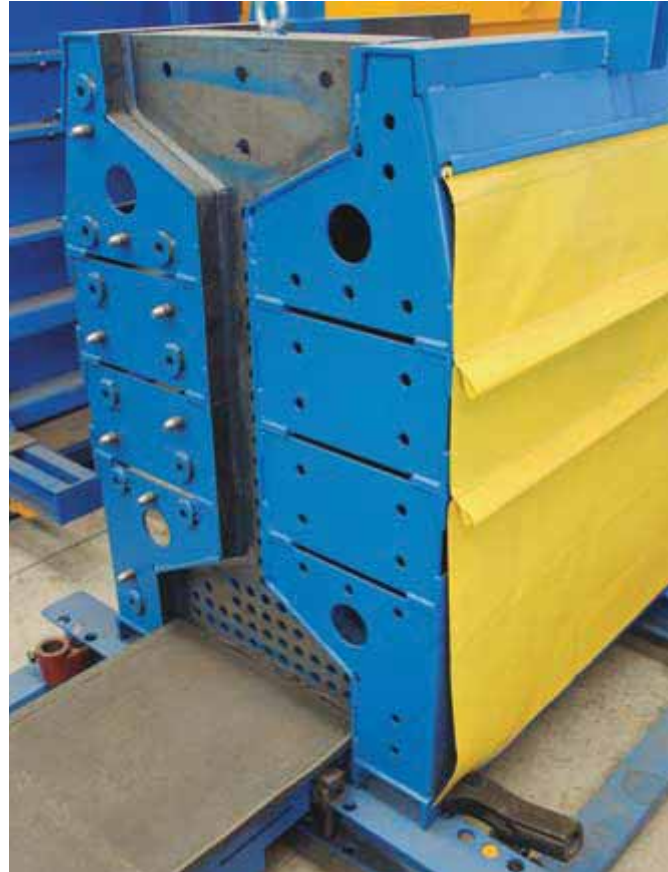
'I' beam mould smould sides with height modulation
