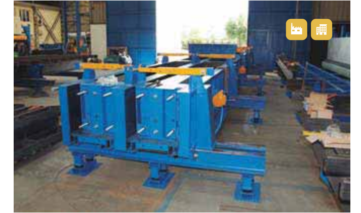
Hydraulic double mould for columns prepared with end stoppers
