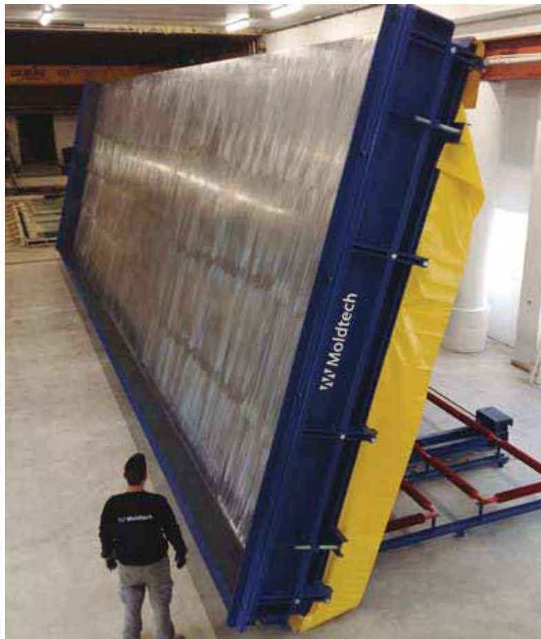
Detail of tilting table with polished surface
