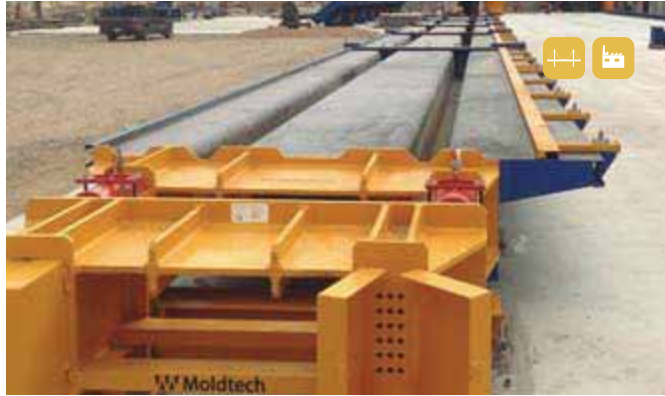
Self supporting TT mould for roofs or pre-slabs of industrial and commercial buildings such as parking garages.
