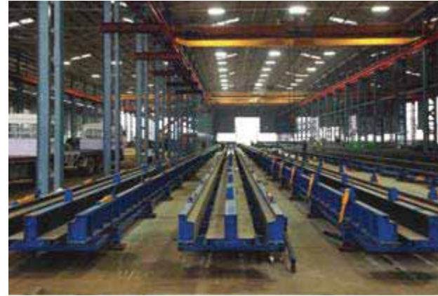
India: complete installation consisting of more than 2km of moulds, for the production of precasted beams used in social housing projects
