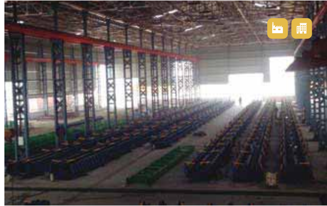
India: complete installation consisting of more than 2km of moulds, for the production of precasted beams used in social housing projects
