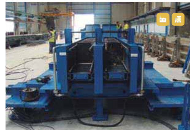
Hydraulic double mould for columns prepared with reinforcement
