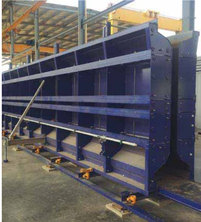
Mould sides for bridge girder
