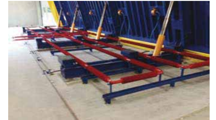
Tilting table with heating on the floor
