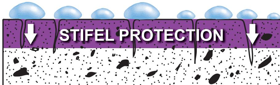
Winter is rough on concrete and rougher still in regions where frequent freeze/thaw cycles are common. If water penetrates the concrete's surface and then changes to ice, the results can be surface scaling. Additionally, corrosive road salts combined with the freeze/thaw cycles can cause untreated surfaces to suffer surface delamination, spalling and scaling.
