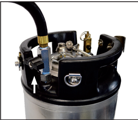
13. Ball valve turned off to prevent product from entering hose and wand assembly.
