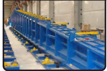
FORMS FOR REINFORCED COLUMNS & BEAMS
