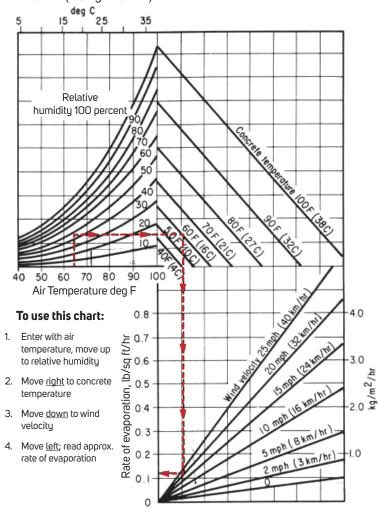
Effect of concrete and air temperatures, relative humidity and wind velocity on the rate of evaporation of surface moisture from concrete. This chart provides a graphic method of estimating the loss of surface moisture for various weather conditions. To use the chart, follow the four steps outlined above. If the rate of evaporation approaches 0.2 lbs/sf/hr (1.0 kg/sm/hr), precautions against plastic shrinkage cracking are necessary. (lerch 1957, ACI 305).
